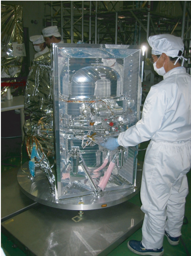
Fig. 18. Finished XRS dewar prior to spacecraft iteration. The rectangular frame attached to the dewar is the radiator close-out panel which fills the gap between the dewar and the spacecraft. The mechanical cooler cold head and compressor are mounted to the upper girth ring.
